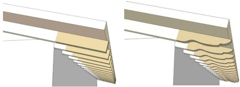
*Why not always use a long rafter end component? Because, in the case of a Hip Roof, some Jack Rafters may be shorter than the end component and won't get cut properly.*
