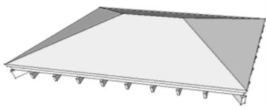
7. A new Roof Style named "New RoofStyle" is added to the "Roof Style" list. Draw another face and select it as in step 1 and choose "Plugins/ Instant Roof/ Make Roof". In the pop-up menu, choose the style we just made, "New RoofStyle" from the "Roof Style?" pull down menu. Choose "yes" for the first option and "no" for the second. Choose "OK".
