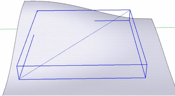
To try out these parameter settings, make a terrain plus a straight line. The terrain must be active and the line must be in a group.
