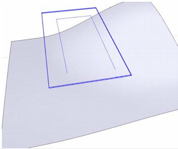
To try out these parameter settings, make a terrain plus a “U” shaped series of lines. The terrain must be active and the lines must be in a group.
