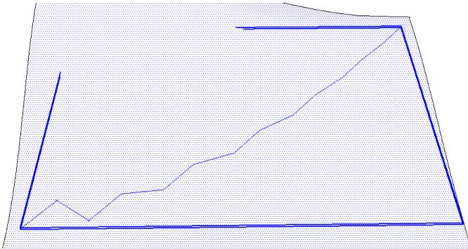
To try out these parameter settings, make a terrain plus a crooked series of lines. The terrain must be active and the lines must be in a group.
