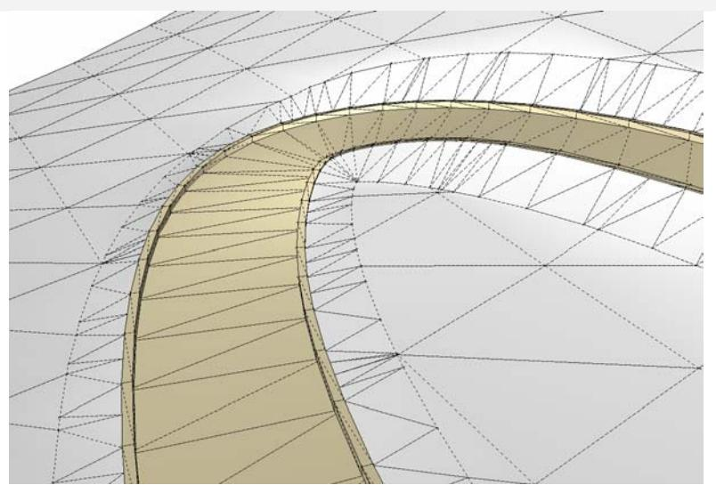
Why not always flatten vertical curves? Because a cross slope can occur when the road is curved - especially if the input value is greater than the width of the road.
