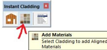
6.3 Materials can be added or changed after the cladding has been modeled. Select the group or groups containing a cladding type, corners, or Mouldings. Then click the Add Materials icon.
