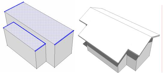
11. For a shed roof, return to step 6. Select the top faces and all but 2 of the top edges as shown. Repeat steps 2 and 3:
