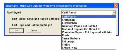
3. Choose "OK" to accept default parameters and generate the roof shown. The next step is to raise the building extension to the correct height. (This is the vertical distance between the top roof planes)
