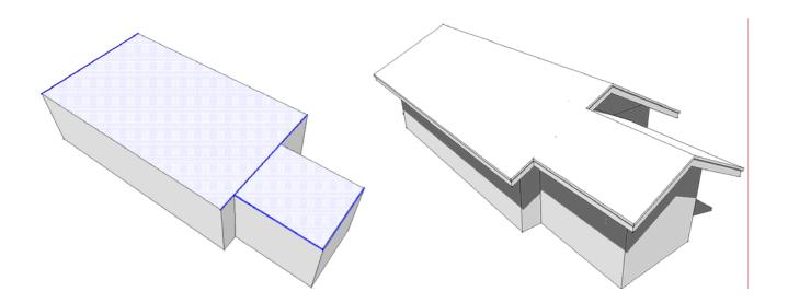
13. *Method 1 - Gable Roof with Continuous Ridge*: Draw geometry similar to below and select all but 2 top edges as shown. Repeat steps 2 and 3 to generate the gable roof:
