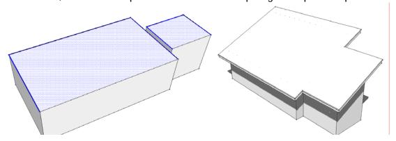
21. For a hip roof, an additional step is required. Use the Push-Pull tool to extend the higher area over the lower as shown. The exact distance is not important. (the extra line can
