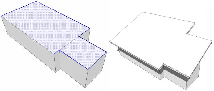
15. *Method 2* - Draw geometry similar to below and select the 6 edges shown. Repeat steps 2 and 3 to generate the gable roof.
