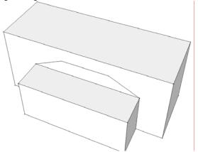
5. Select the lower face. Use the move tool to raise the face by the distance between the top of the gable wall outline to the upper face. (Inference-lock the z axis)
