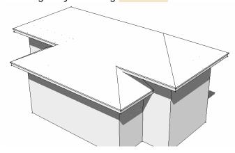
10. For a hip roof, return to step 6. Select the top 2 faces and the 5 edges shown. Repeat steps 2 and 3:
