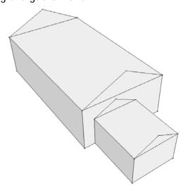
17. Select the lower face. Use the move tool to raise the face by the distance between the lower face and the top of the upper triangular gable wall directly above. (Inference-lock the z axis)
