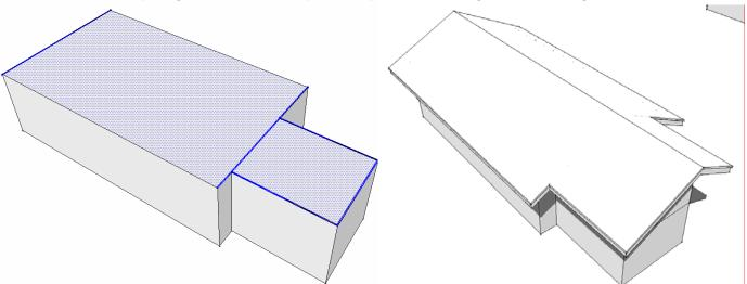
14. *Method 1- Shed Roof*: Draw geometry similar to below and select the edges as shown. Repeat steps 2 and 3 to generate the shed roof:
