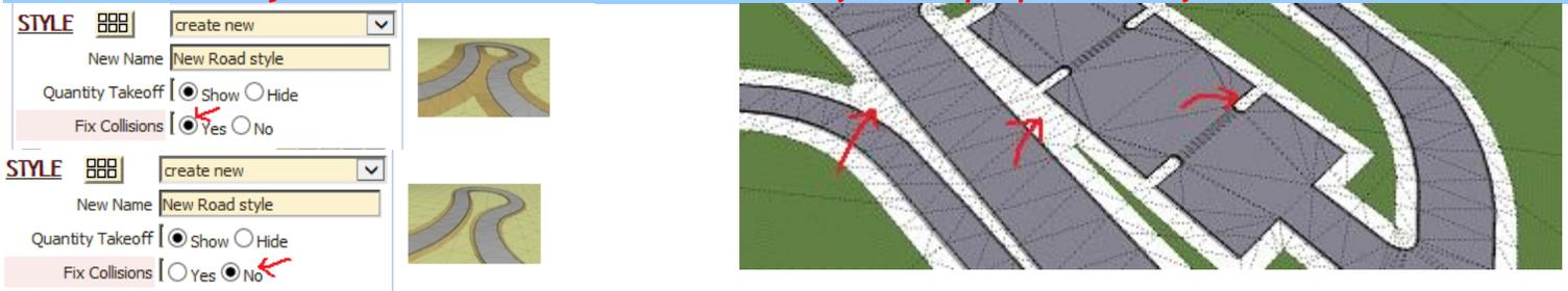
**Method for Road from Centerline** *Road from Center Line* can have trouble making the road surfaces when there are small segments in the input curve. Use the 'Meticulous' setting to resolve a highly detailed road from centerline input. Note that this method is slower than the Standard method.
