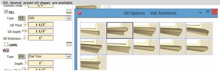
Like the custom surround, to use a custom profile for your sill, draw a 2d profile in the xy plane and save it as a component. The easiest way is to
